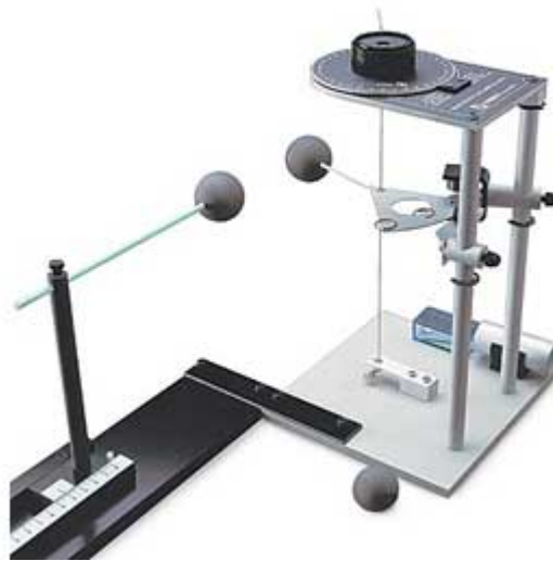
Figure 4.1.: Coulomb's Law apparatus
