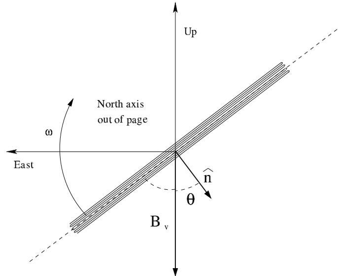
Figure 8.2.: Definition of angles for flux through rotating coil.
