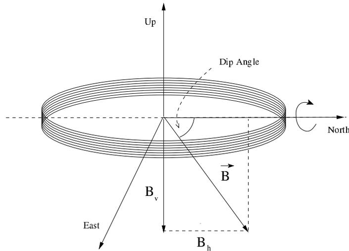
Figure 8.3.: Rotating coil magnetometer directly measuring vertical component of Earth's magnetic field.
