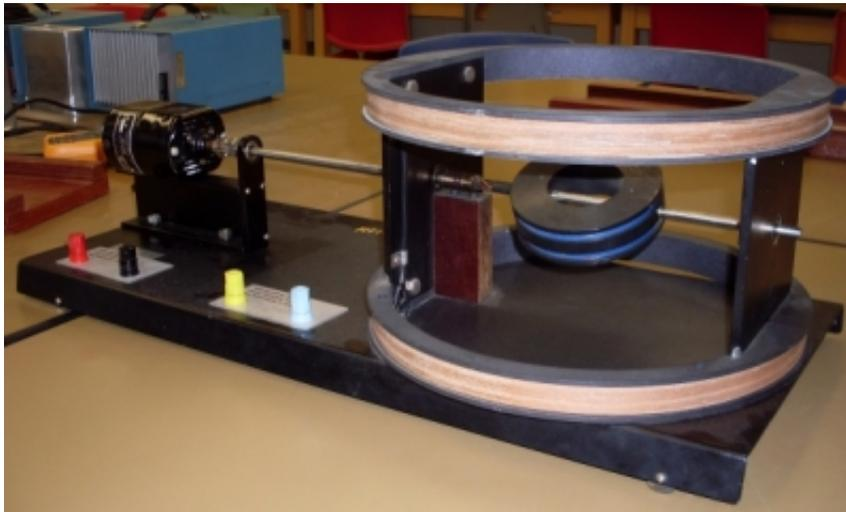
Figure 8.1.: Rotating coil magnetometer showing motor, rotating coil and Helmholtz coils.
