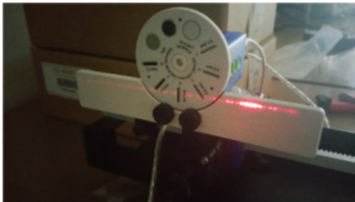
Figure 11.3.: Single slit pattern projected horizontally onto aperture bracket
