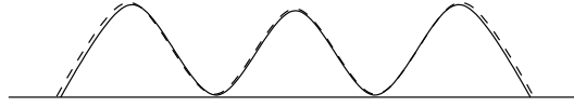
Figure 2.2.: Two fringe patterns overlapping to produce strong fringes. Note the dashed line is of slightly longer wavelength.
