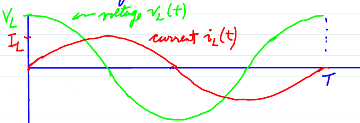
Figure 5: Current i_L(t) lags applied voltage v_L(t) for an inductor.
